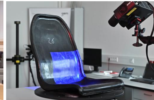
Seat Measurement using GOM
