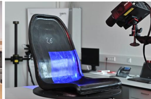
Seat Measurement using GOM
